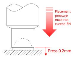
Figure 17. Placement pressure due to placement depth
