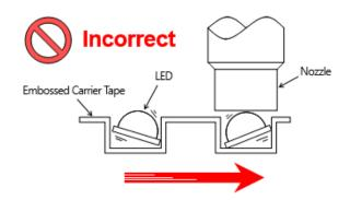
Figure 11. Tape feeder feed rate (fast)
