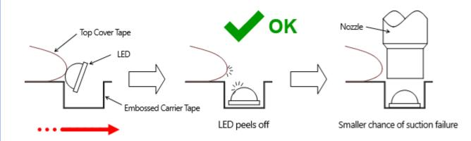
Figure 14. When the tape feeder feed rate is slow and the LED sticks to top cover tape
