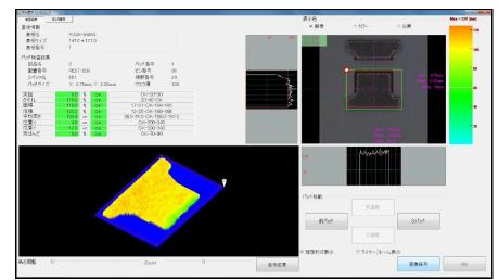
Figure 3. Example of the data for a visual inspection after solder printing (Reference: CKD VP6000M-V)
