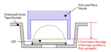
Figure 7. Recommended nozzle height (example: part number NFxW585AR Assembly Precaution application note)
