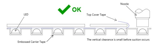
Figure 16. Removing the top cover tape just before suction
