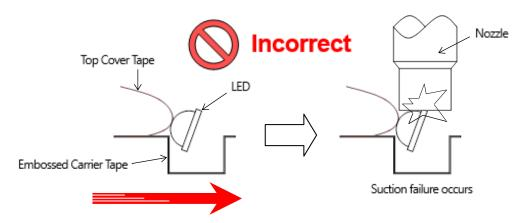
Figure 13. When the tape feeder feed rate is fast and the LED sticks to top cover tape
