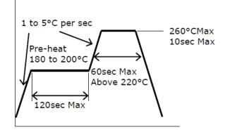
Figure 19. Recommended Reflow Soldering Condition (example: part number NFSW757H-V1 Specification)
