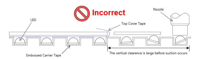
Figure 15. Removing the top cover tape in the normal position
