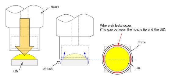
Figure 8. Air leak at the time of LED suction (example: part number NV9W149AM)
