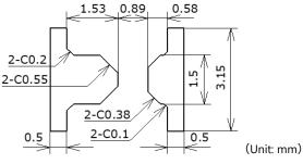
Figure 2. Example metal solder stencil aperture as a countermeasure against part floating
