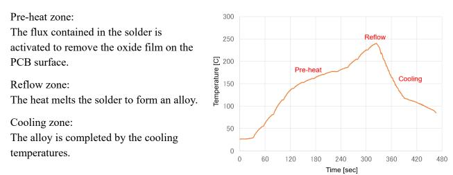
Figure 20. Example of a Reflow Profile
