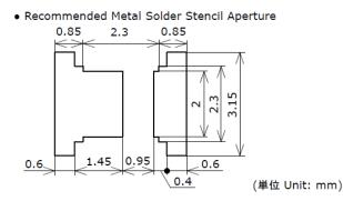
Figure 1. Recommended soldering pad pattern and recommended metal solder stencil aperture (example: part number NFSW757H-V1 Specification)
