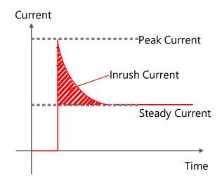
Figure 24. Example of an inrush current waveform
